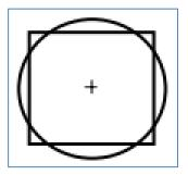
The more material is spread out, the stronger the column.
